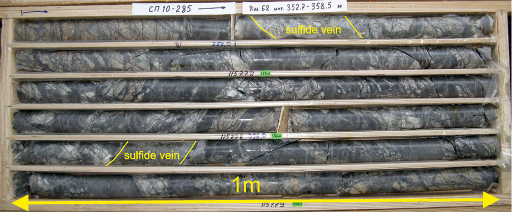
Fig. 19. Intense, but sulfide-free and barren, quartz stockwork veining at the foot-zone of the Peschanka orebody. Rare late-stage sulfide veins cut the quartz stockwork.
